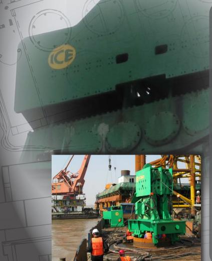
Patented Dual-pull<sup>™</sup> suppressor provides maximum vibration isolation during driving and light extraction combined with high pull capability for tough extraction jobs.
