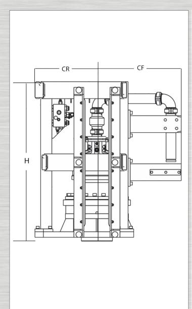
Angle guides for 26" (660 mm) leads. Optional guides for leads side-mount or H-Beam available.
