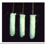
**Above:** Three model bored piles from the U of Houston Study poured aftrer 24 hrs. of excavation open time show perfect geometery.
