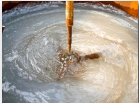
Circular Slurry Mix Tank showing Slurry thickening, or Yielding while being Stirred, or Agitated with Paddle Mixer
