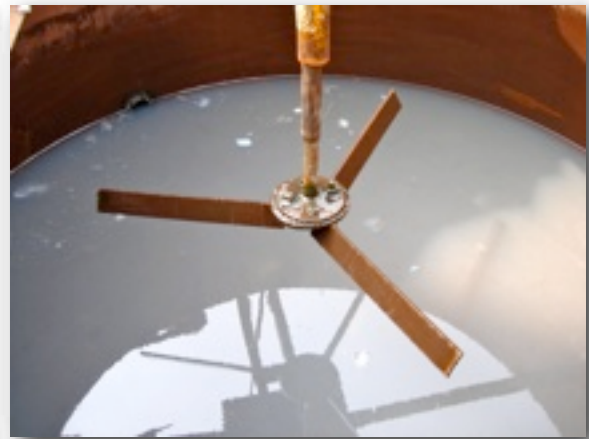
Circular Slurry Mix Tank showing Paddle Mixer Blades
