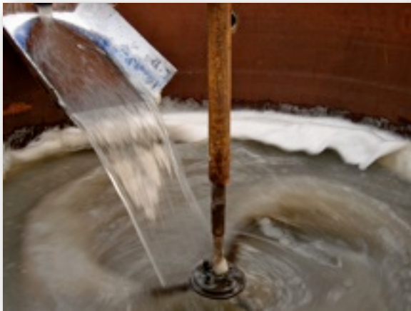
Circular Slurry Mix Tank showing Slurry Filling Tank and being Stirred, or Agitated with Paddle Mixer
