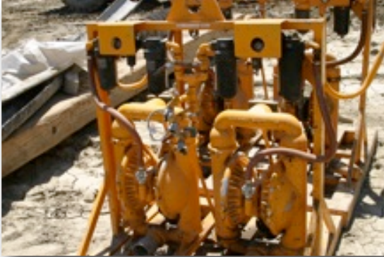
Double Diaphragm Pumps Setup in Tandem for Rapid Slurry Supply on Large Excavation
