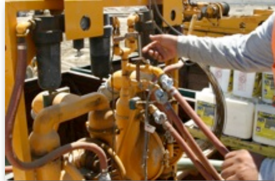
Double Diaphragm Pumps Setup in Tandem for Rapid Slurry Supply on Large Excavation
