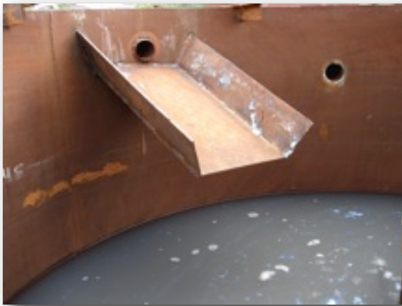
Circular Slurry Mix Tank showing Splash Pan
